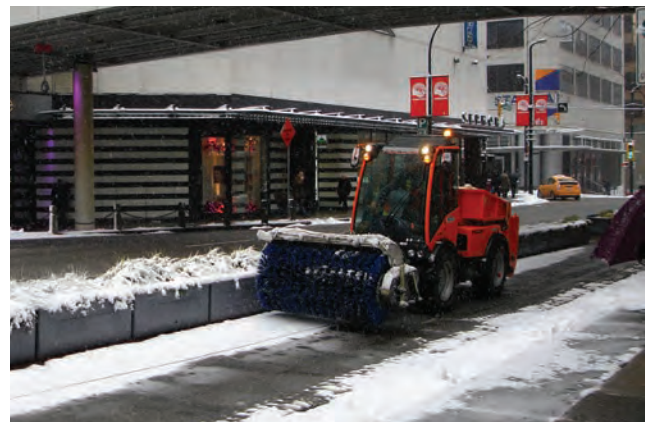
Figure 64: A vehicle specially designed to clear snow from bicycle facilities in Vancouver, British Columbia
