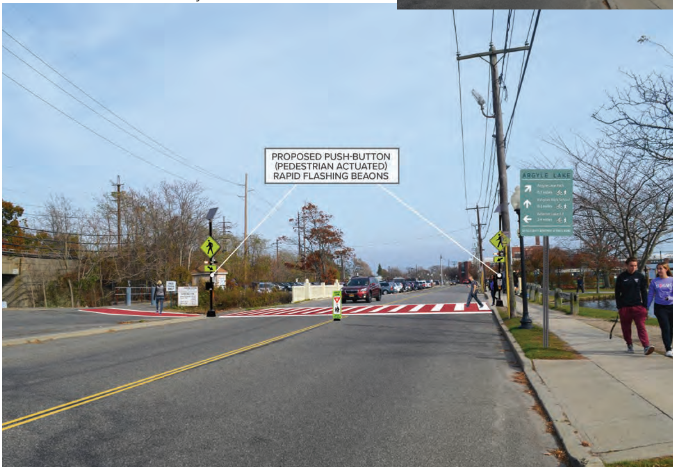
Figure 52: This photo simulation shows a proposed pedestrian crossing with RRFB's on Trolley Line Road in Babylon
